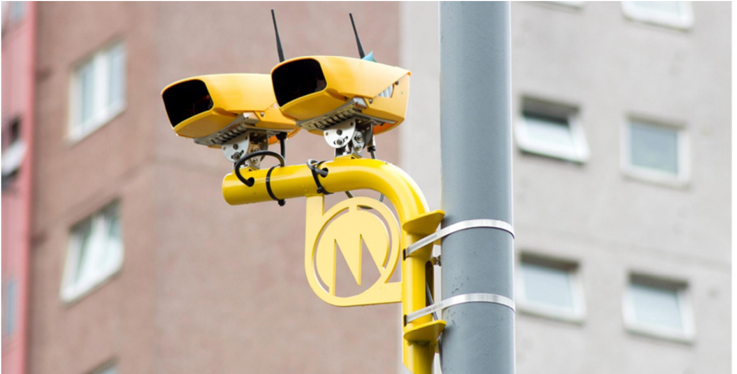
Low cost, spot speed replacement SPECS installation using highly distinctive street lighting brackets (West Midlands).
