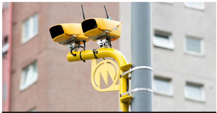
Low cost, spot speed replacement SPECS installation using highly distinctive street lighting brackets (West Midlands).
