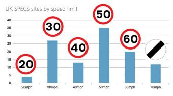
SPECS is successfully used with every speed limit, demonstrating the same level of casualty reduction on all road types. Over 700km of UK roads are under permanent average speed control currently, in addition to the 400+temporary roadworks sites that have been operated.
